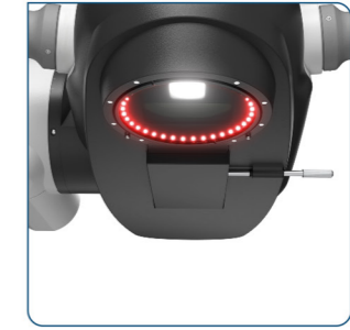
The fully integrated keratoscope provides a quick assessment of the corneal curvature.
